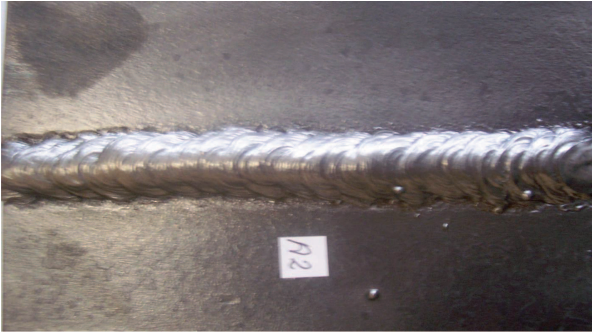
Fig. 1. The general view of welded AISI 1030 steel couples
