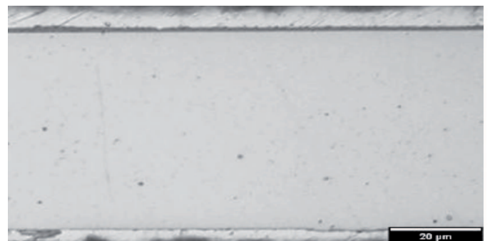
Fig. 6. High-temperature superconducting tape of SF series, magnification 500x
