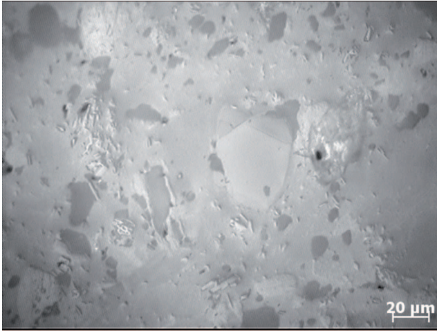
Fig. 4. Representative structure of the sample loaded up to the early subcritical stage of degradation, magnification 500x. Dark areas remaining after crushed out particles of cullet and quartz grains constitute about 4% of the surface. Fine bright grains of corundum and grey mullite precipitates are not affected by degradation
