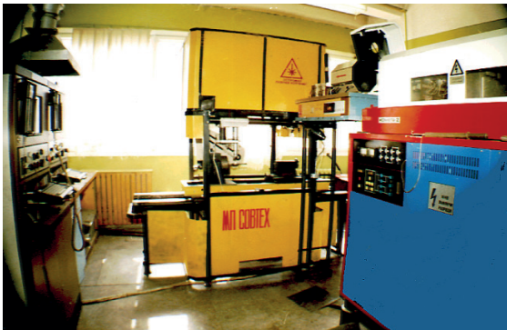
Fig. 2. Test stand of the laser hardening „Kometa-UNILAM” [22]
