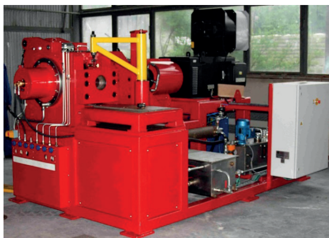
Fig. 2. A Conform-type device for the continuous rotary extrusion
