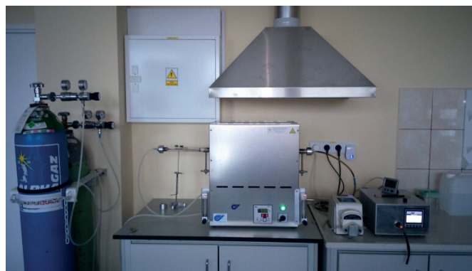
Fig. 1. Research stand for measuring the gas evolution rate of materials (acc. to Method 1), Laboratory of Environmental Protection
