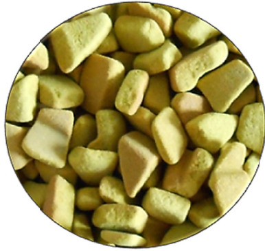
Fig. 3. Precursors – the Croning technology
