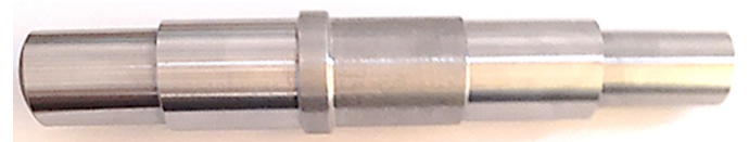
Fig. 1. The specimen processed by turning
