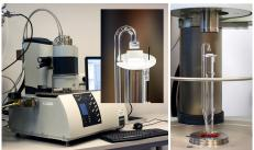
**TMA 402 F1 Hyperion, NETZSCH:** useful sample dimensions: length 0.01 to 20 mm, diameter 1 - 10 mm. Starting length of the sample determined automatically. Load in the range ± 3N, increase in 1 mN steps . Resolution of the deformation - 0.125 nm in the range of 5000um. Temperature range
