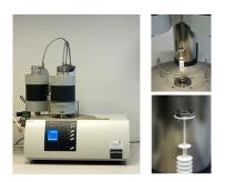
DSC 404 F1 Pegasus, NETZSCH: flux type calorimeter, temp. -170 - +1000 °C (steel furnace) and
