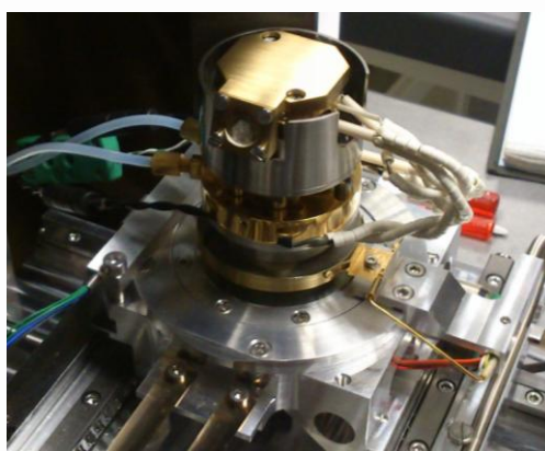
Fig.6. Pretilted SEM heating stage for EBSD application.
