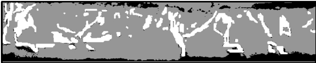
Fig. 5. The structure analysis area for the computation of the volumetric Si fraction of the Al-Si coating the Image ProPlus 30 for Windows software
