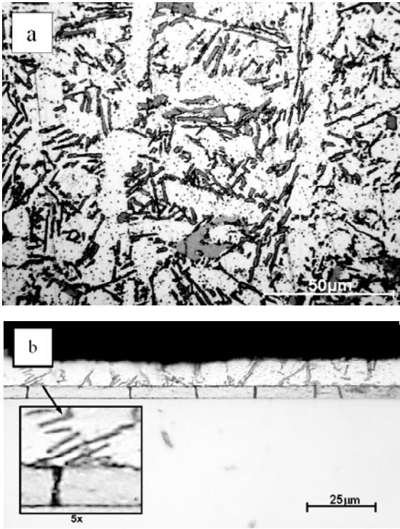
Fig. 1. Microstructures of the initial coating, a) in parallel plane to the substrate of the metal sheet, b) on the cross section of the coat, etched by 1%HF
