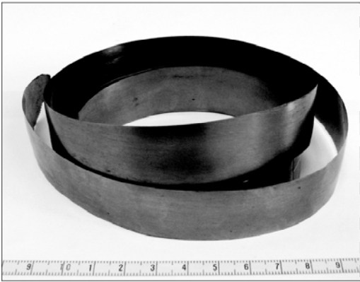
Fig. 7. Thin, high strength Ni 3 Al (Zr, B) strip (0.08mm x 25mm x 2800mm) obtained by author’s technology
