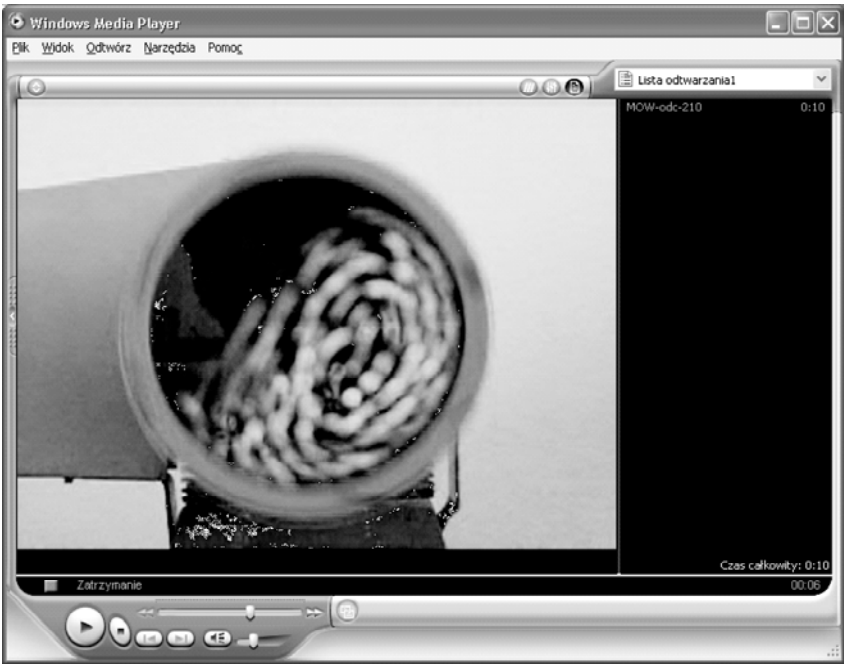
Fig. 9. Instantaneous position of balls in the rotary-vibrational mill chamber – during operation in the Department of Manufacturing Systems AGH
