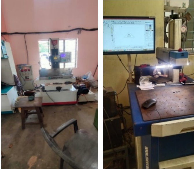
Fig. 4. Electric Discharge Drilling (EDD) and LASER source
