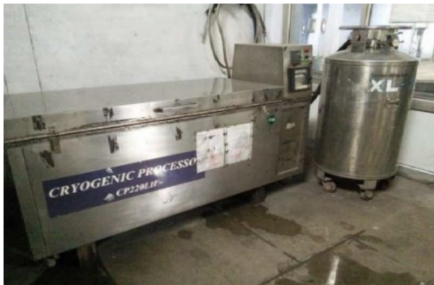
Fig. 9. Cryogenic setup for treatment of cutting inserts
