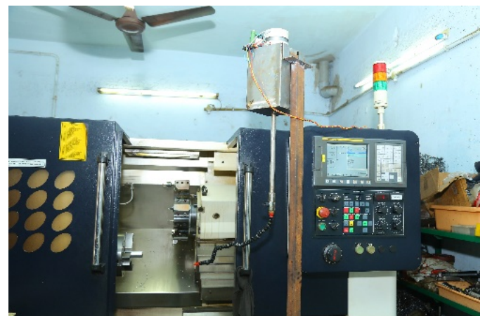
Fig. 7. CNC setup with solid lubrication supply system
