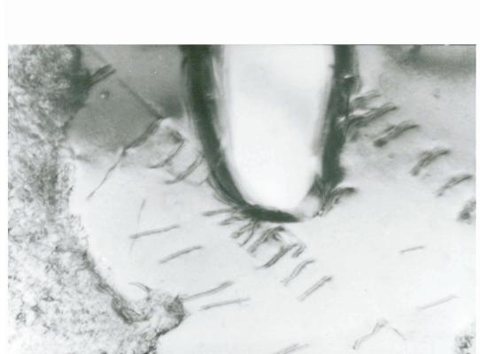
Fig. 4. Microscopic image of phase boundary in  $\text{Ni}_3\text{Al}/\text{TiB}_2$  composite. Note well visible dislocations present in the matrix material
