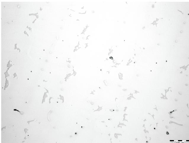
Fig. 22. Microstructure of the Ni<sub>3</sub>Al /TaB composite surface, 100x
