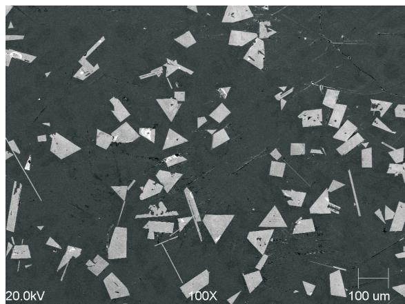
Fig. 10. Scanning image of Ni<sub>3</sub>Al/WC composite. 100x
