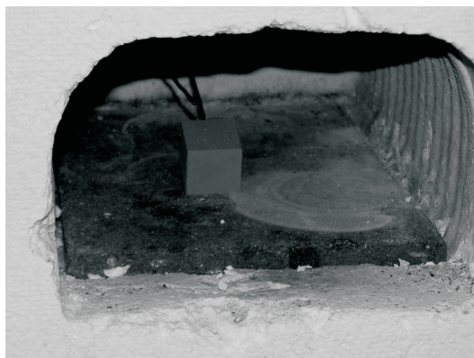
Fig. 3. The exemplary cubic sample with a thermocouple of type K (on the left) and muffle furnace with the 8-channel temperature recorder (on the right)
