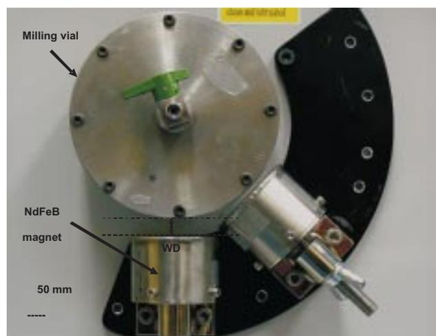
Fig. 1. Angular positions of Nd-Fe-B super-strong magnets for ball milling under high energy impact mode in the Uni-Ball-Mill
