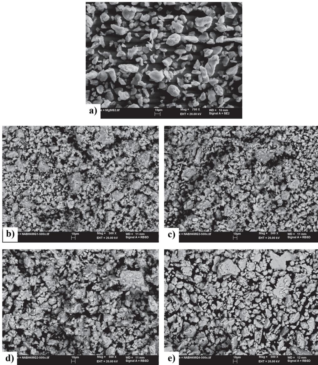
Fig. 4. SEM micrographs of (a) as received Mg powder and the composite powders after ball milling for (b) NaBH<sub>4</sub> + 8 vol.% Mg, (c) NaBH<sub>4</sub>+43 vol.% Mg, (d) NaBH<sub>4</sub>+63 vol.% Mg, (e) NaBH<sub>4</sub>+87 vol.% Mg
