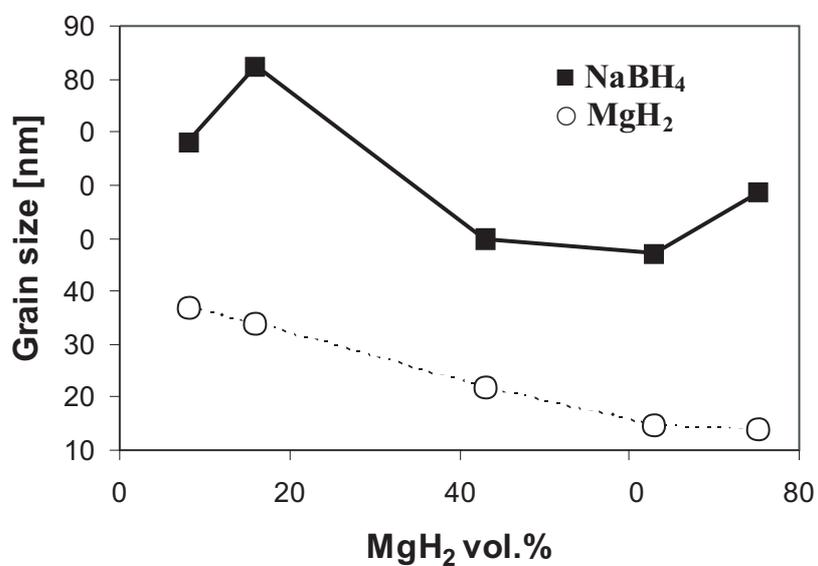
Fig. 6. Grain size of NaBH<sub>4</sub> and MgH<sub>2</sub> after ball milling as a function of MgH<sub>2</sub> content in the (NaBH<sub>4</sub>+MgH<sub>2</sub>) composites
