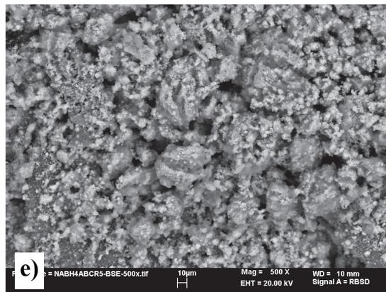
Fig. 2. SEM micrographs of the as received powder of (a)  $\text{NaBH}_4$  and (b)  $\text{MgH}_2$ , and the composite powders after ball milling for (c)  $\text{NaBH}_4+8\text{vol.}\% \text{MgH}_2$ , (d)  $\text{NaBH}_4+16\text{vol.}\% \text{MgH}_2$  and (e)  $\text{NaBH}_4+43\text{vol.}\% \text{MgH}_2$
