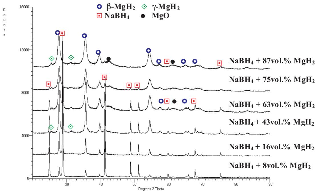
Fig. 5. XRD patterns of the (NaBH<sub>4</sub> + MgH<sub>2</sub>) composites
