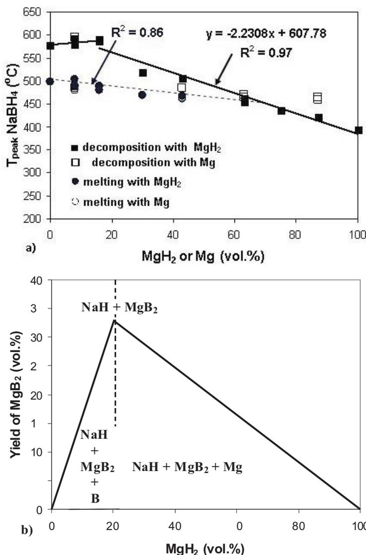
Fig. 9. The influence of MgH<sub>2</sub> content on the destabilization of NaBH<sub>4</sub> – (a) the NaBH<sub>4</sub> decomposition and melting DSC peak temperatures as a function of MgH<sub>2</sub> content; (b) The theoretical yield of MgB<sub>2</sub> formation for NaBH<sub>4</sub> + MgH<sub>2</sub> reaction as a function of MgH<sub>2</sub> content. Adopted from [5]
