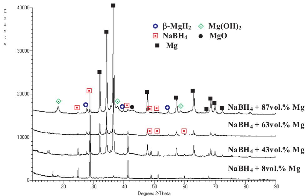
Fig. 7. XRD patterns for NaBH<sub>4</sub> composites
