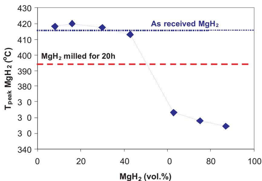
Fig. 11. The  $\text{MgH}_2$  decomposition DSC peak temperatures as a function of  $\text{MgH}_2$  content in the  $(\text{NaBH}_4 + \text{MgH}_2)$  composites
