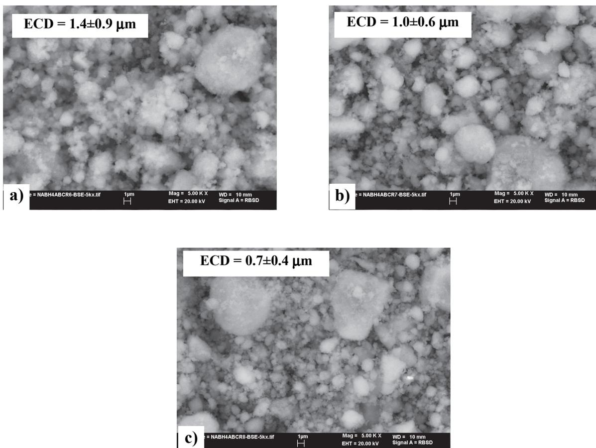
Fig. 3. SEM micrographs of composite powders after ball milling for (a)  $\text{NaBH}_4+63$  vol.%  $\text{MgH}_2$ , (b)  $\text{NaBH}_4+75$  vol.%  $\text{MgH}_2$  and (c)  $\text{NaBH}_4 + 87$  vol.%  $\text{MgH}_2$
