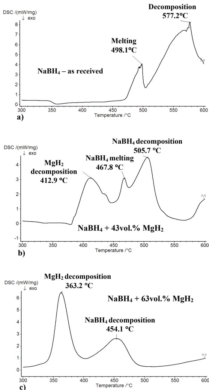
Fig. 8. DSC curves for (a)  $\text{NaBH}_4$  as-received, (b)  $\text{NaBH}_4 + 46$  vol.% $\text{MgH}_2$  and (c)  $\text{NaBH}_4 + 63$ vol.%  $\text{MgH}_2$  composites
