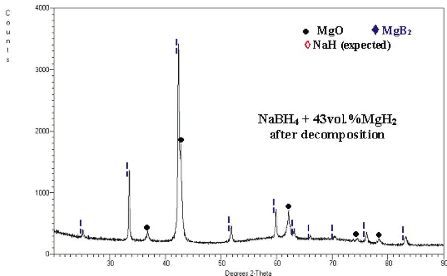
Fig. 10. XRD patterns for  $\text{NaBH}_4 + 43\text{vol.}\% \text{MgH}_2$  composite after decomposition at  $600^\circ\text{C}$
