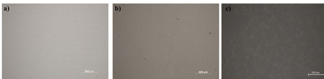
Fig. 3. Results of microscopic observation of a) Ti_is, b) Ti_sg, c) Ti_ald, after pitting corrosion tests
