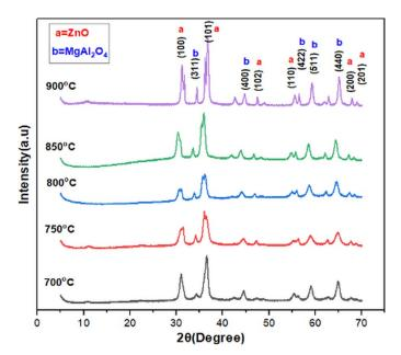
Fig. 1. The XRD pattern of  $ZnO-MgAl_2O_4$  sample at different annealing temperature
