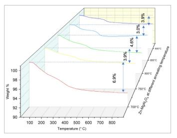
Fig. 2. The TGA curve behaviour for samples at different annealing temperature
