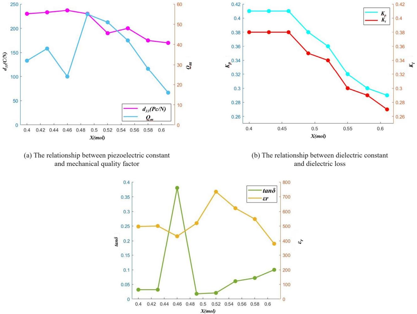
Fig. 4. Electrical Properties of  $K_xN_{1-x}N-LN$  Ceramics
