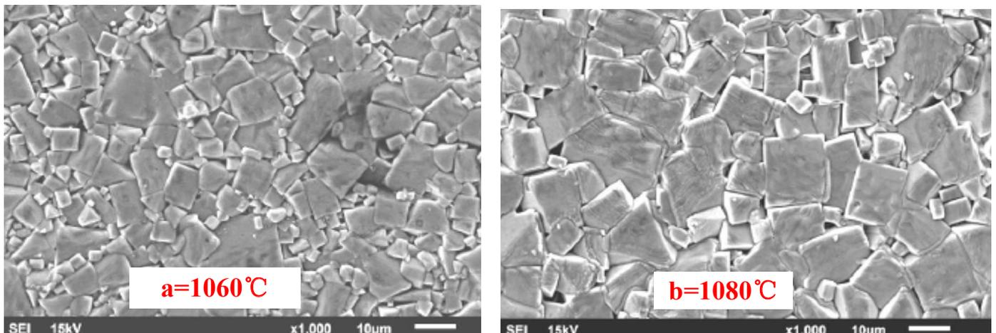
Fig. 3. SEM images of KNN-LN ceramic surface at different sintering temperatures
