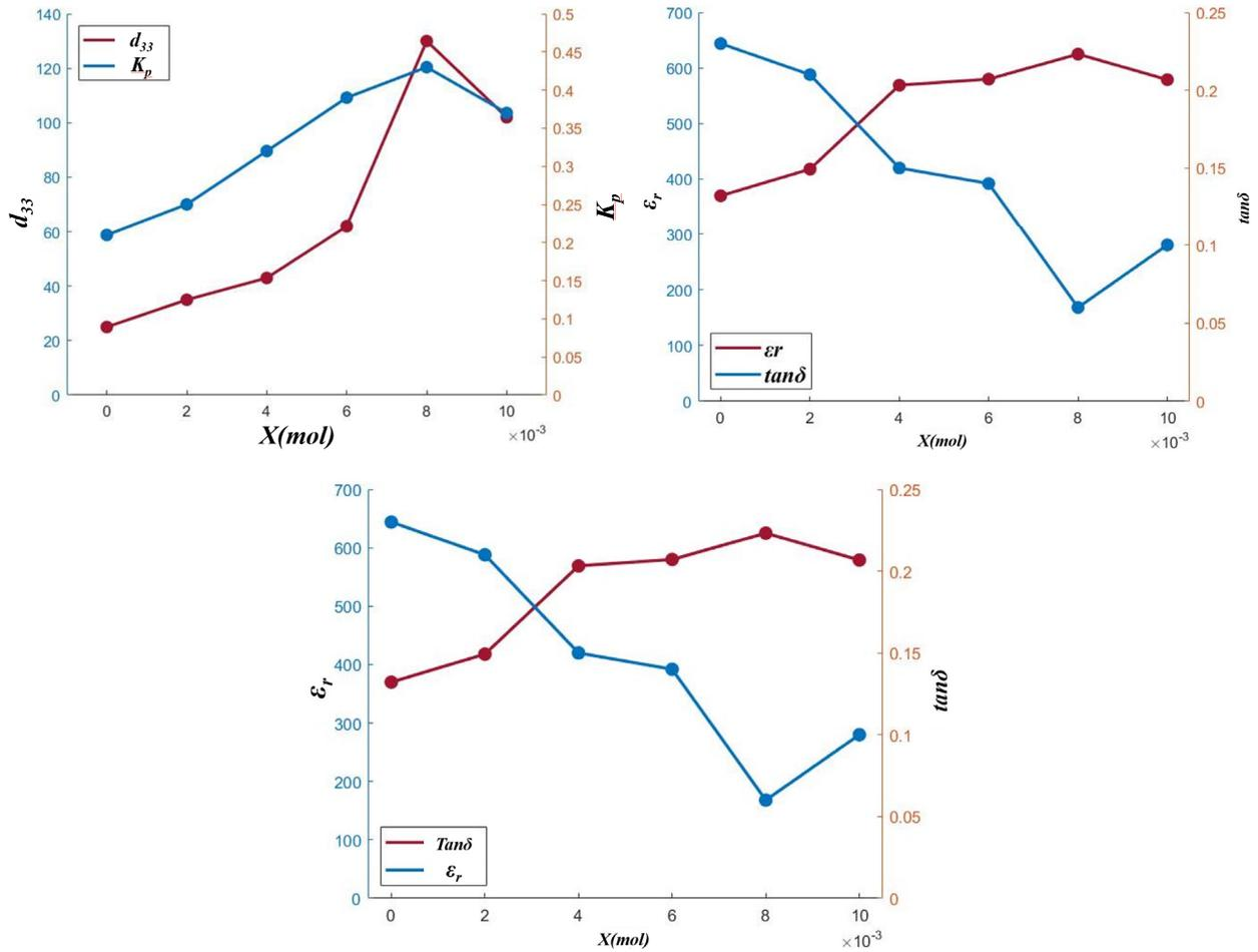
Fig. 5. Analysis of the Electrical Properties of KNN-yBF Ceramics
