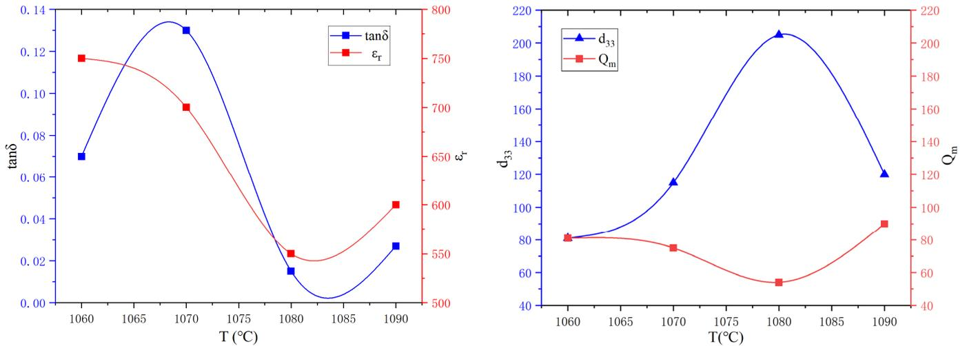
Fig. 2. The Influence of Sintering Temperature on the Electrical Properties of KNN-LN Ceramics
