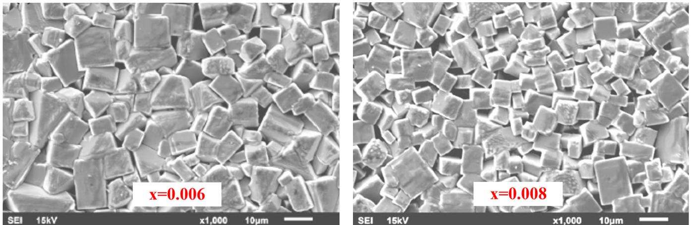
Fig. 6. SEM images of ceramic surfaces at 1100°C with different BF dosages
