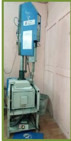
Fig. 1. Ultrasonic cavitation with stir-casting setup [31]
