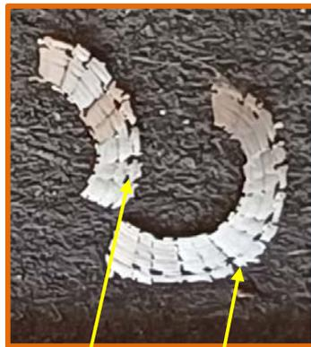
Short very thin shaped curled chip with cracks & voids
