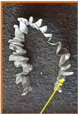
Continuous thin shaped chip with lamella structure
