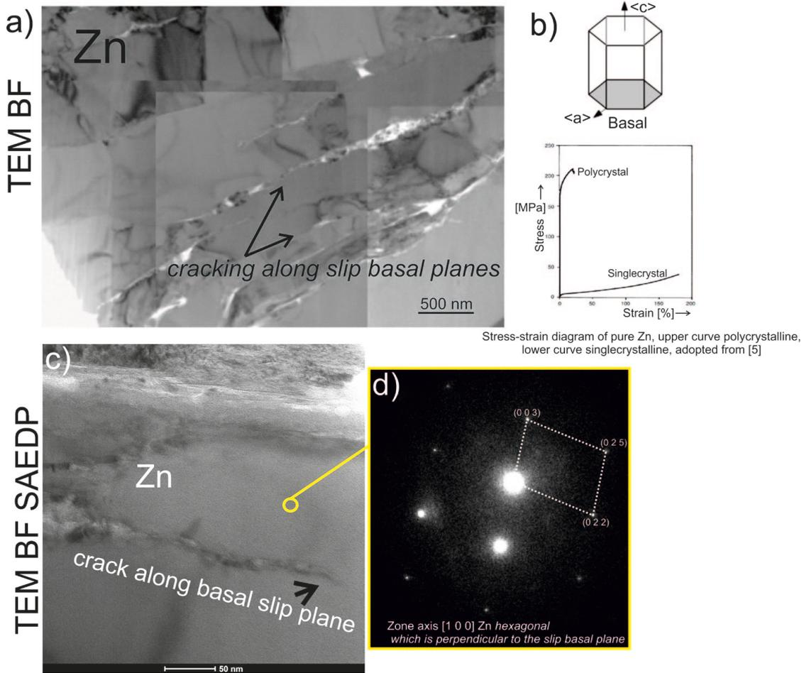
Fig. 5. Microstructure characterization of the cracking process in the Zn phase in the uploading process during wear done by TEM BF; a). TEM BF image of the cracking process in Zn phase; b). scheme of crystallographic planes along which cracking appeared and illustration of the tensile test of polycrystalline Zn as well as single crystalline phase; c). TEM BF of the cracks (higher magnification); d). SAEDP of the Zn phase
