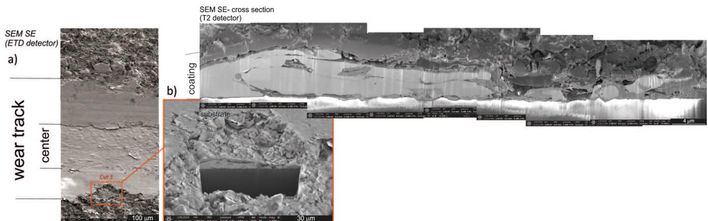
Fig. 1. Topography image done by SEM (SE) of wear track with indicated area for the following TEM characterization; a). plan view of the wear track; b). cross-section of the wear track
