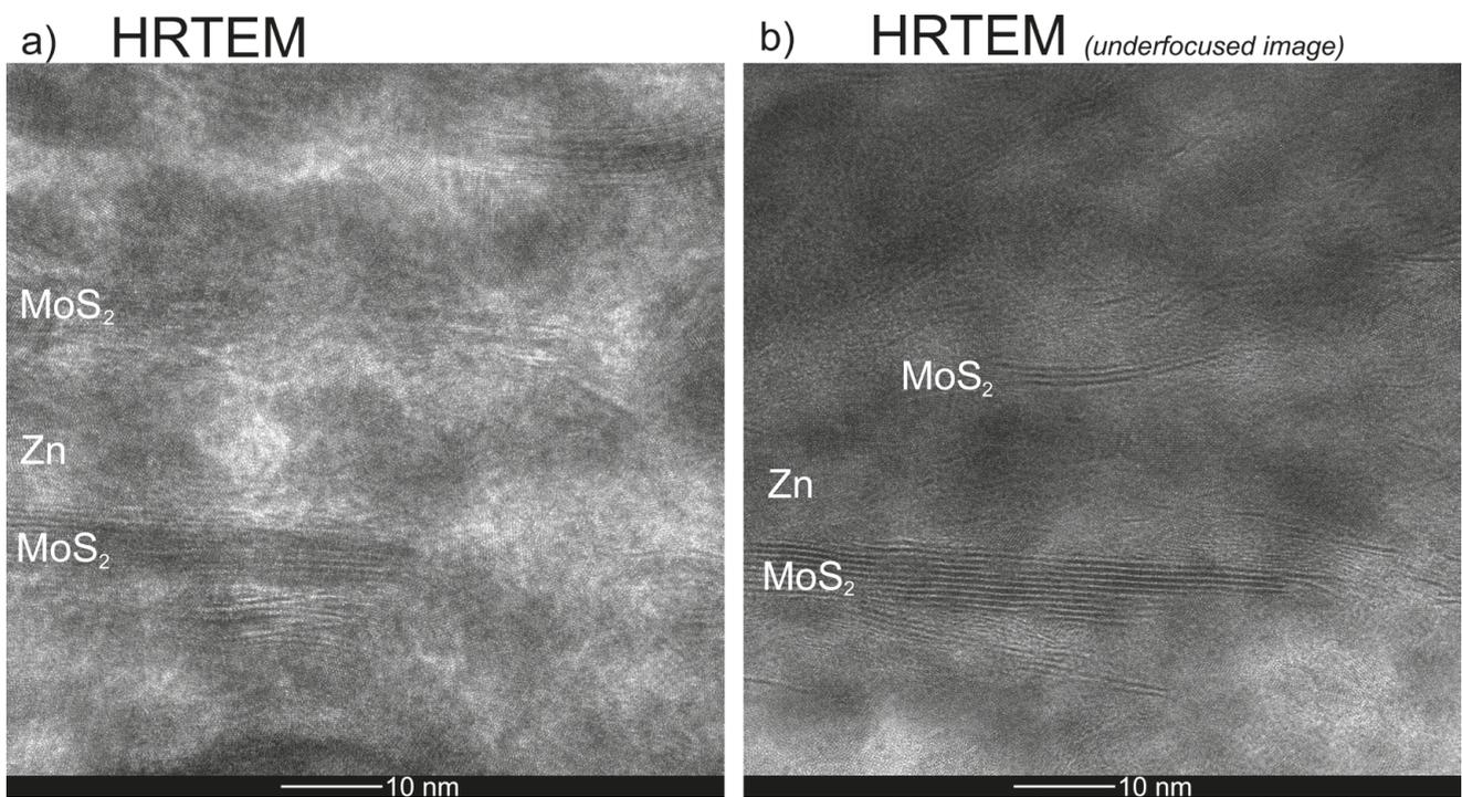
Fig. 10. The HRTEM analysis of the coating from the wear center on the cross-section
