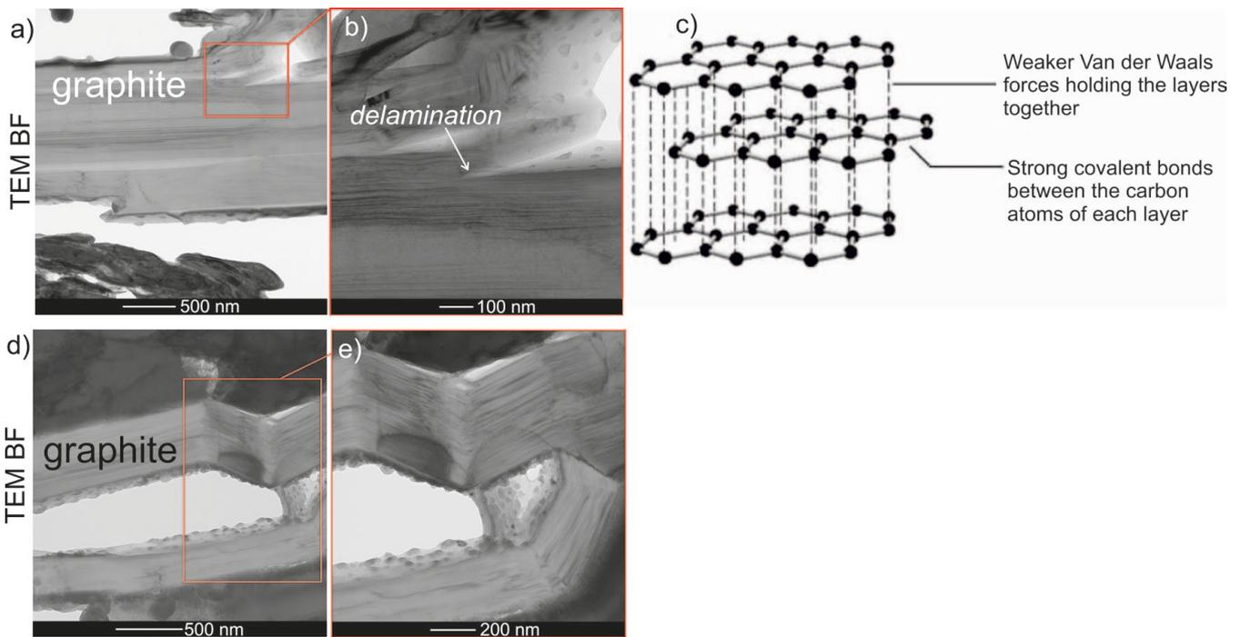
Fig. 3. Microstructure characterization of the wear mechanism in the graphite phase; a). TEM BF image of the wear mechanism in the graphite phase; b). higher magnification; c). scheme of the graphite atomic layers arrangement; a). TEM BF image of the kinking deformation in the graphite phase; b). higher magnification of the kinking deformation effect
