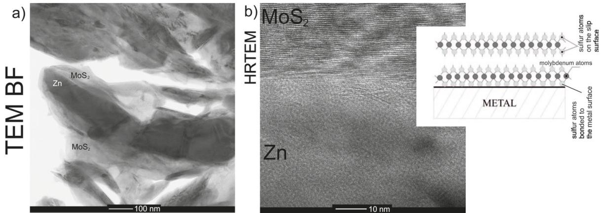
Fig. 7. Microstructure characterization of self-healing effect on the cross-section; a) TEM BF image; b) HRTEM image together with the scheme of the atomic layers arrangement in the MoS<sub>2</sub>
