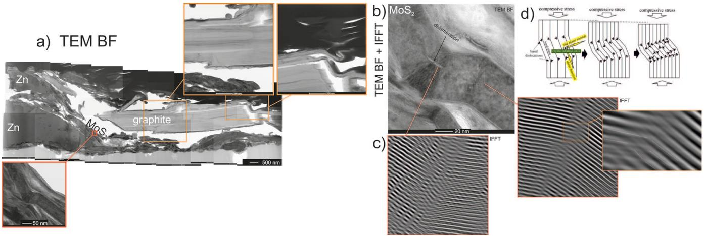
Fig. 2. The cross- section analysis of the coating close to the wear track done; a) TEM BF of the coating on the cross-section; b). TEM BF image of the kinking deformation mechanism; c). IFFT image; d). scheme of the kinking deformation
