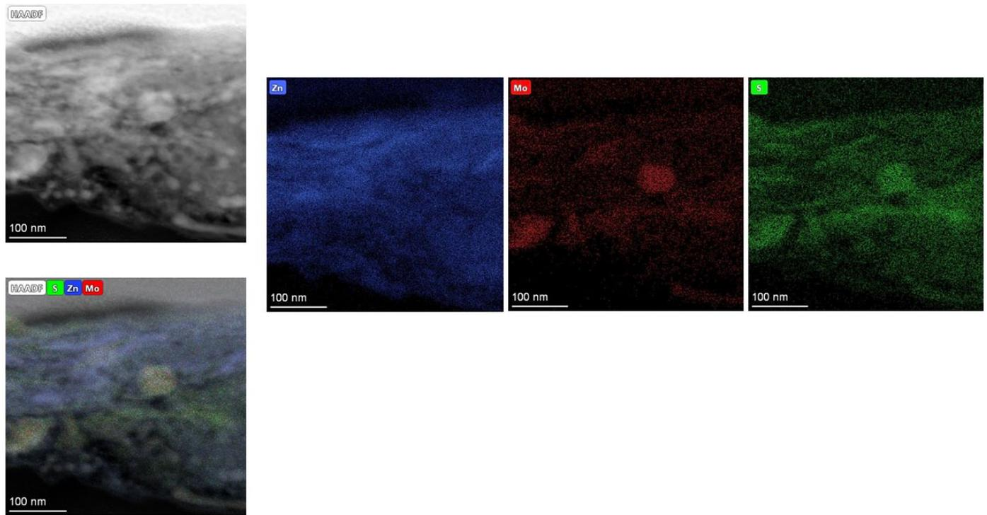
Fig. 9. Qualitative chemical analysis of the coating from the center of the wear path done by STEM and EDS
