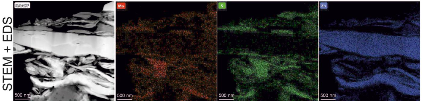
Fig. 6. Qualitative chemical analysis of the coating on the cross-section done by STEM and EDS
