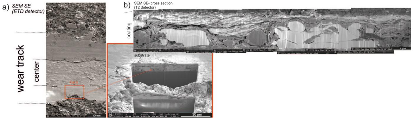
Fig. 4. a). Topography image of wear track with indicated area for the following TEM characterization; b). cross section characterization done by SEM (SE)
