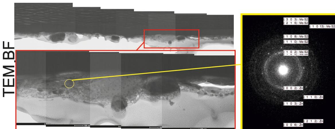
Fig. 8. Microstructure characterization of the coating from the center of the wear path on the cross-section done by TEM BF; a) TEM BF image of the coating on the cross-section; b) SAEDP
