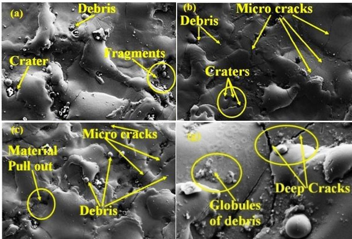
Fig. 8. SEM graphs of Inconel 800 specimen machined by PMEDM
