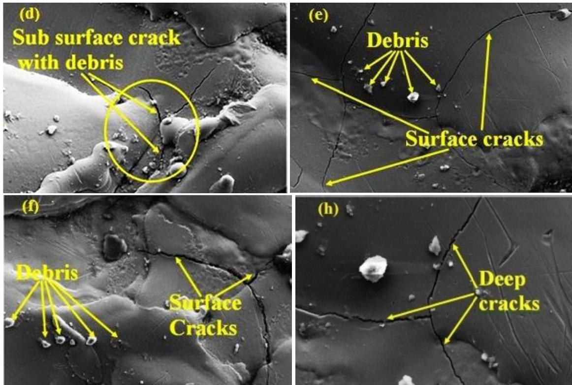
Fig. 9. SEM graphs of Inconel 800 specimen machined by EDM
