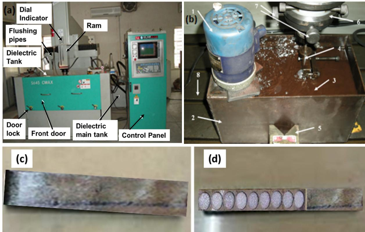
Fig. 1. EDM machine and specimen used in this study: (a) during machining by EDM; (b) pictorial view of used EDM machine; (c) specimen before machining; and (d) specimen after machining
