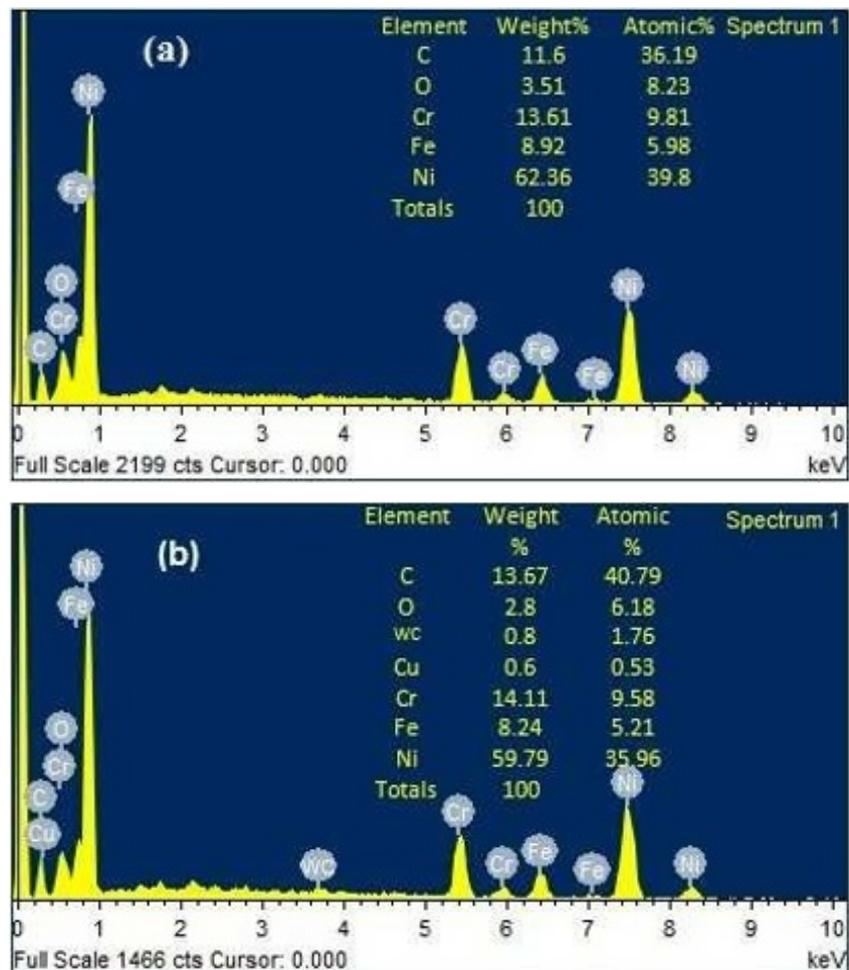
Fig. 10. EDX analysis of specimen machined by EDM and PMEDM using identical paraments: (a) EDM: and (b) PMEDM
