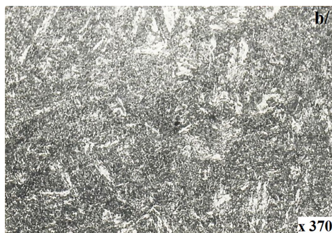
Fig. 1. Microstructure of the tested steel (×370): a/ as received; b/ quenching; c/ annealing at 200°C; d/ annealing at 600°C
