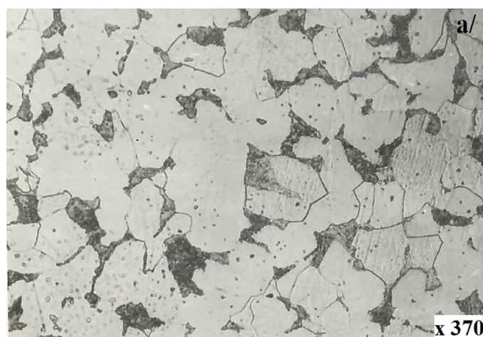
Fig. 1. Microstructure of the tested steel (×370): a/ as received; b/ quenching; c/ annealing at 200°C; d/ annealing at 600°C
