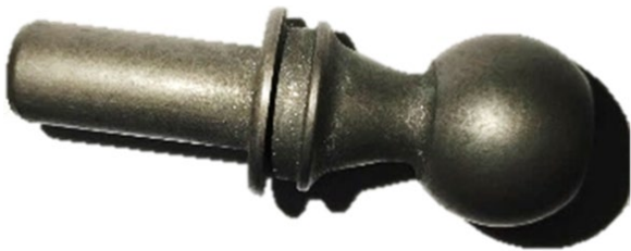
Fig. 2. Machined prototype of the stabilizer link with spherical element
