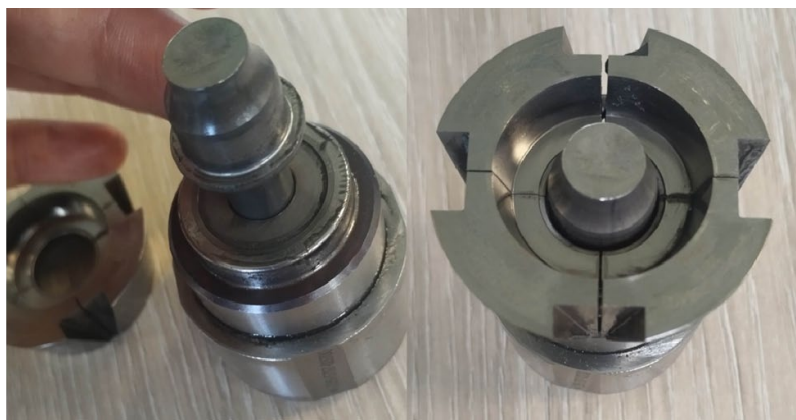
Fig. 8. Segmented die with the shaped preform installed in the die sleeve
