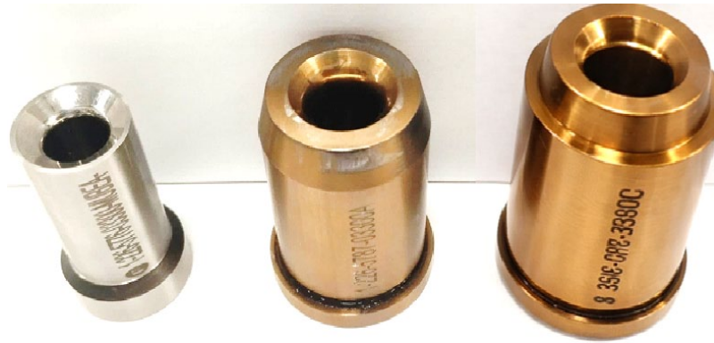
Fig. 14. Modification of the bushing supporting the upper head in Operation IV of Variant II: original (100 bolts), first modification (10,000 bolts), final design (100,000 bolts)
