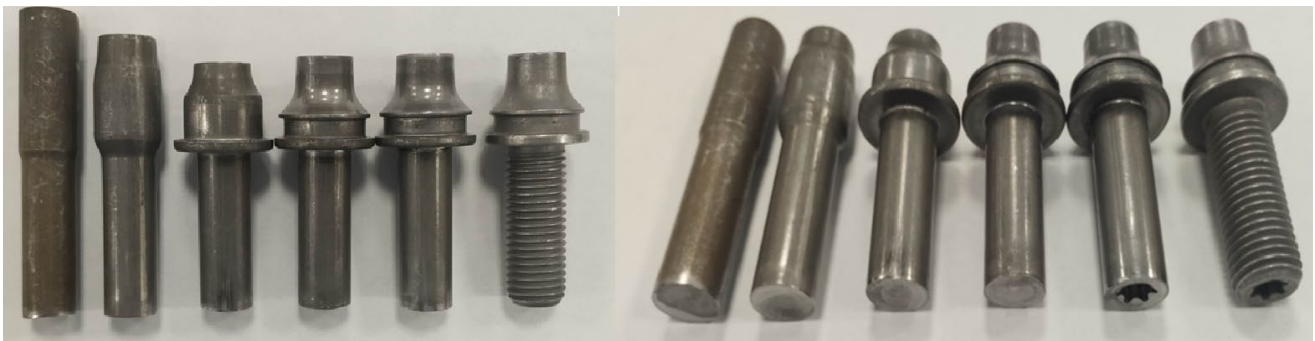
Fig. 9. Preforms shaped in Variation II of the technological trials
