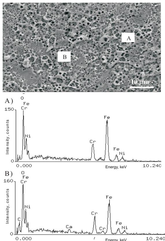
Fig. 4. Topography of austenitic steel after LSP, 2 shots (SEM SE), the EDS spectra show presence of oxygen, iron, chromium and nickel at the treated surface
