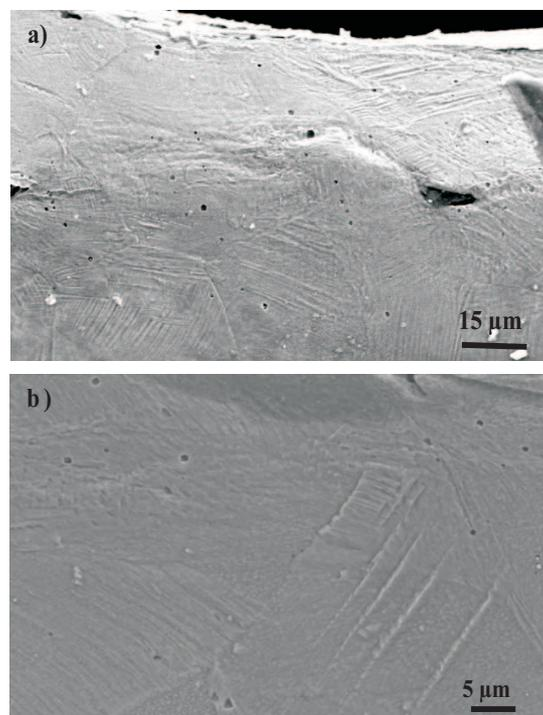
Fig. 5. Slip bands on the cross section of the treated surface; SEM, a) low magnification, b) high magnification
