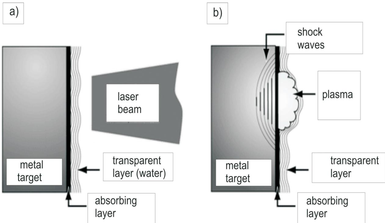
Fig. 1. Schematic representation of the laser shock processing (a) metal target with absorbing and water layers (b) shock wave generation by laser beam
