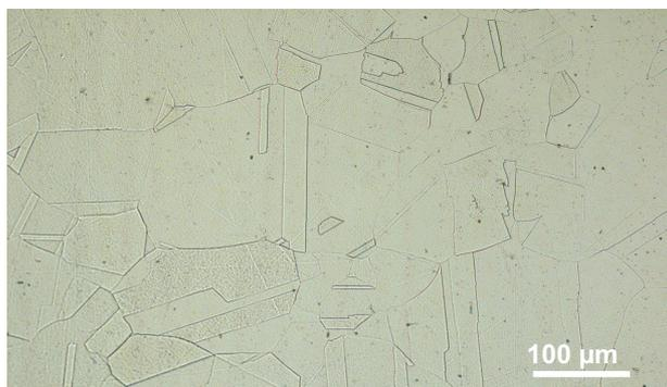
Fig. 3. Microstructure of austenitic stainless steel before the laser treatment (light microscopy)
