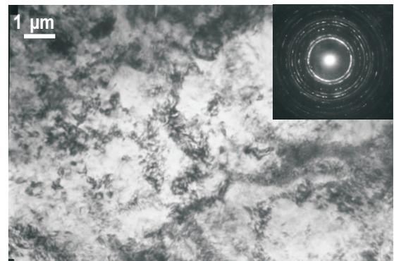
Fig. 7. High density of dislocations in the LSP treated austenitic stainless steel with corresponding diffraction pattern
