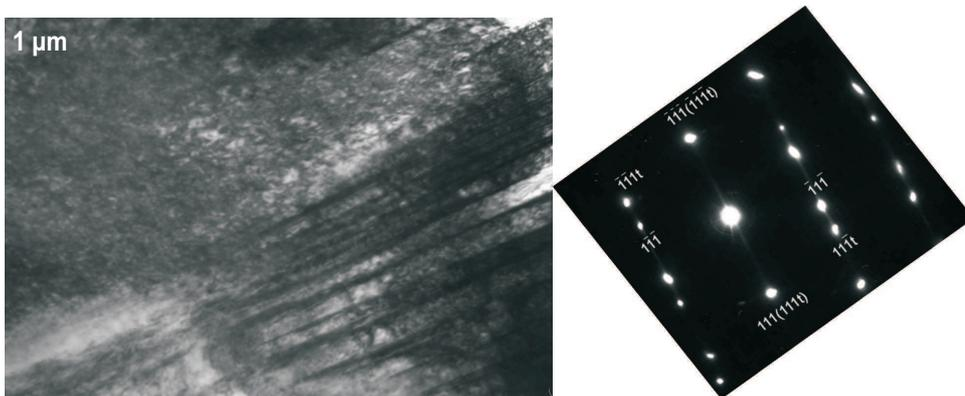
Fig. 8. Deformation twins in the LSP treated austenitic stainless steel with corresponding diffraction pattern
