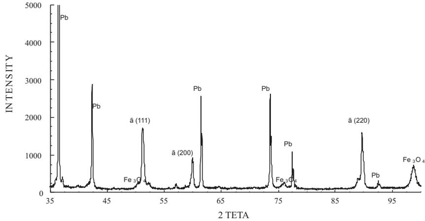
Fig. 6. XRD pattern of austenitic stainless steel after LSP ( $C_{\alpha}K_{\alpha}$  radiation)
