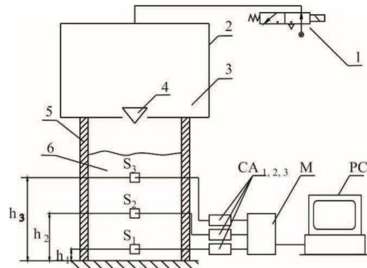
Fig. 4. Layout of test stand for examining impulse compaction of moulding sands and measuring circuit: 1 - distribution valve, 2 - impulse head, 3 - accumulator tank, 4 - impulse valve, 5 - moulding box, 6 - moulding sand,  $S_{1,2,3}$  - piezoelectric sensors Kistler type 601A,  $CA_{1,2,3}$  - charge amplifier Kistler type 5015A, M - data acquisition module Keithley KUSB 3100, PC - computer
