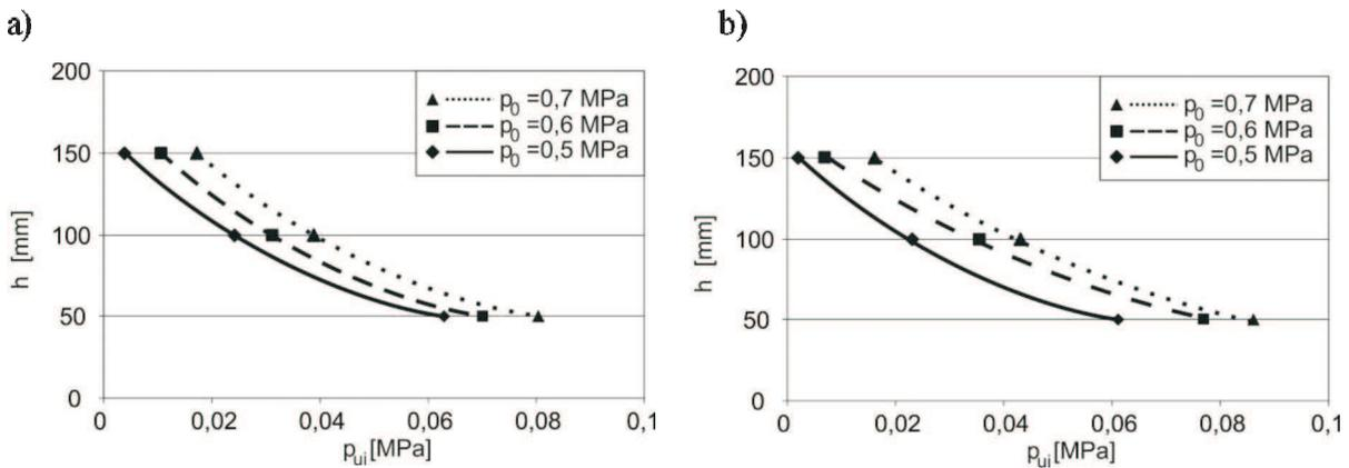
Fig. 8. Changes of pressure  $p_{ui}$  in function of sandmix column height for initial compressed air pressures  $p_0 = 0.5; 0.6; 0.7$  MPa: simulation results (a) and experimental results (b)
