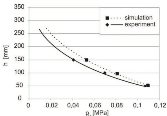
Fig. 10. Changes of pressure  $p_{ui}$  in function of height of the sandmix column for initial compressed air pressure  $p_0=0.6\text{MPa}$  and height of the moulding box  $H_2=350\text{mm}$ : simulation results and experimental results
