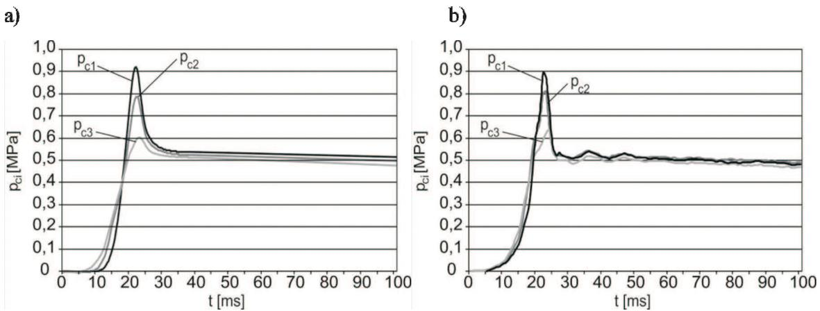
Fig. 7. Changes of total pressure  $p_{ci}$ : simulation results (a) and experimental results (b) for the moulding sand with 6% of bentonite and humidity  $W=3.5\%$
