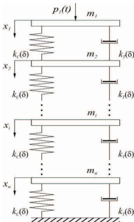
Fig. 3. Laminar rheological model of moulding sand
