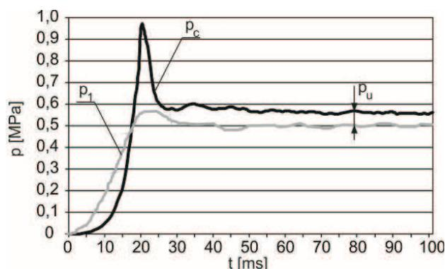
Fig. 2. Stepwise characteristics of moulding sand with 5% of bentonite and humidity  $W=2.5\%$
