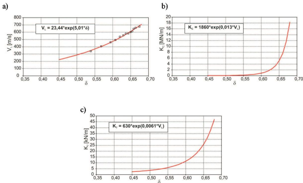
Fig. 5. Measurement results of ultrasonic wave speed  $V_L = f(\delta)$  (a) as well as relationships  $k_C = f(\delta)$  (b) and  $k_T = f(\delta)$  (c) for moulding sand with 5% of bentonite and humidity  $W=2.8\%$
