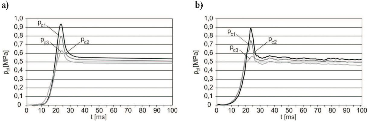
Fig. 6. Changes of total pressure  $p_{ci}$ : simulation results (a) and experimental results (b) for the moulding sand with 6% of bentonite and humidity  $W=2.8\%$
