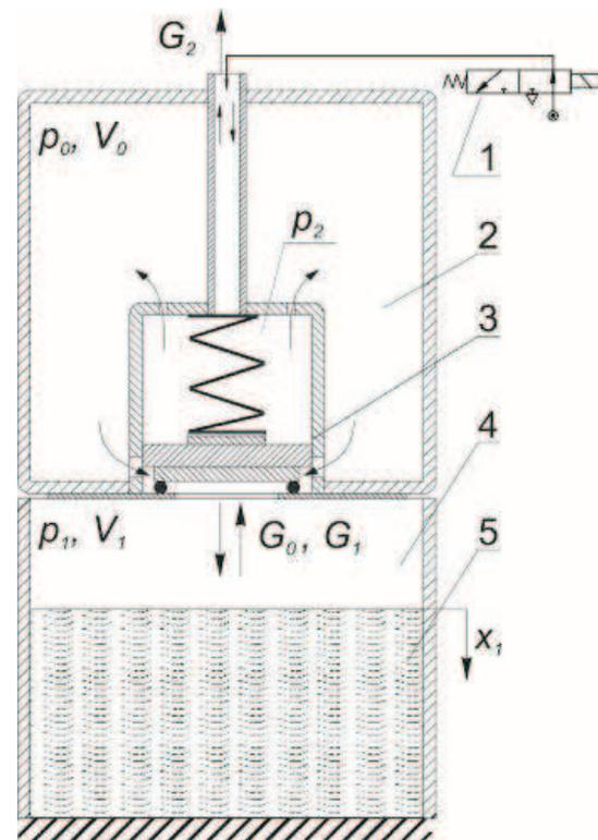
Fig. 1. Layout of the impulse compacting head, controlled by a self-acting impulse valve: 1 - distribution valve; 2 - accumulator tank; 3 - self-acting impulse valve; 4 - technology space; 5 - moulding sand,  $p_i$  - absolute pressure in  $i^{\text{th}}$  chamber,  $G_i$  - outflow rate from  $i^{\text{th}}$  chamber,  $V_i$  - capacity  $i^{\text{th}}$  chamber,  $x_i$  - coordinate of top layer of compacted sandmix column
