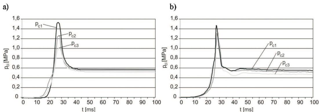
Fig. 9. Changes of total pressure  $p_{ci}$ : simulation results (a) and experimental results (b) for initial compressed air pressure  $p_0=0.6\text{MPa}$  and height of the moulding box  $H_2=350\text{mm}$
