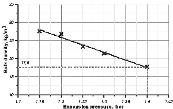
Fig. 6. Influence expansion pressure on the density of foamed polystyrene at constant time t=180 s
