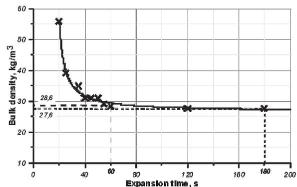
Fig. 5. Influence expansion time on the density of foamed polystyrene at constant pressure  $P=1.15$  bar
