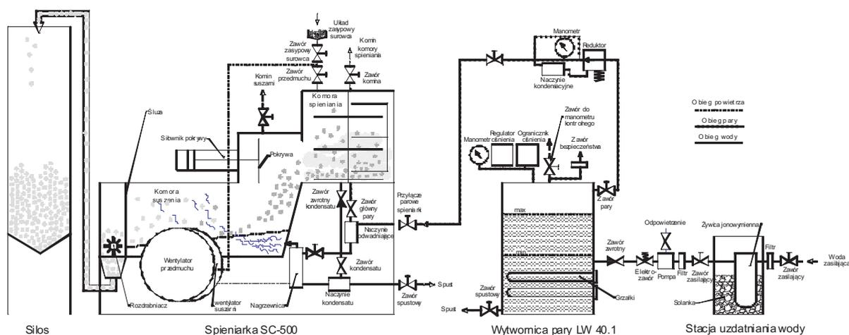
Fig. 3. Scheme station of pre-expansion the polystyrene, equipped with a batch pre-expander. [11]
