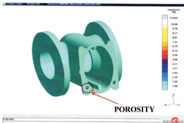
Fig. 6. One of the possible places of porosity occurrence in cast valve body determined by numerical computations
