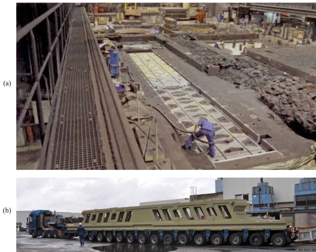
Fig. 11. Giant iron casting of a two-piece machine bed manufactured at Siempelkamp Giesserei GmbH (Krefeld, Germany): sand-mold preparation process (a) and the finished casting ready for transport (b).
