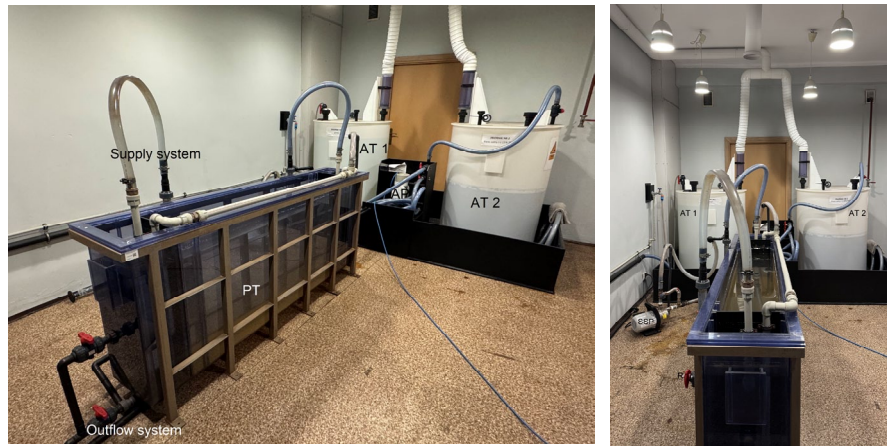
Fig. 3. Physical model of the pickling tank with flow control infrastructure and acid tanks (AT – acid tanks, PT – pickling tank, AP – acid pump, SSP – supply system pump, R - rotameter)
