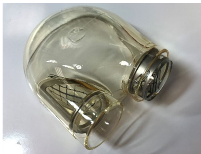
Fig. 4. The primary purpose of oligoproline coatings. Intended for use on the blood-carrying chamber of a pneumatic cardiac assist device. The image shows a modified chamber developed as part of the project No. M-ERA. NET/2014/01/2016, “Nonthrombogenic metal-polymer composites with adaptable micro and macro flexibility for the next generation heart valves in artificial heart devices”
