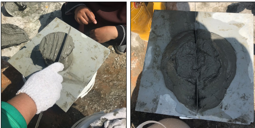
Fig. 2. Spreadability test executed on each fresh LFC-PFF hybrid mix
