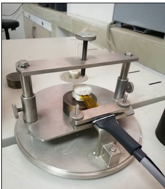
Fig. 3. Setup for thermal test
