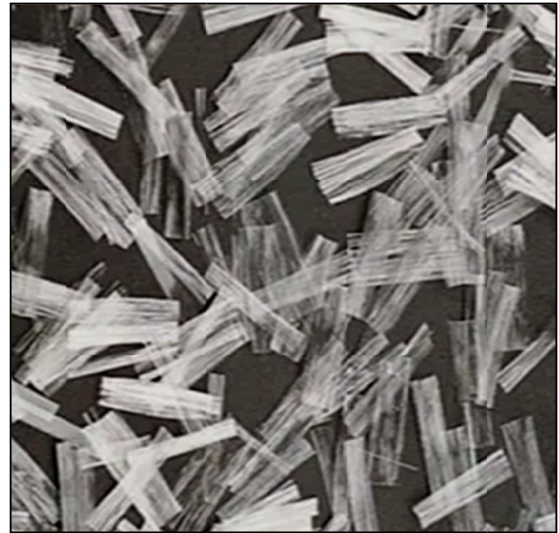
Fig. 1. Polypropylene fibrillated fibre (PFF) utilized in this study
