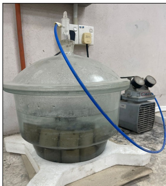
Fig. 4. Permeable porosity test via vacuum saturation technique
