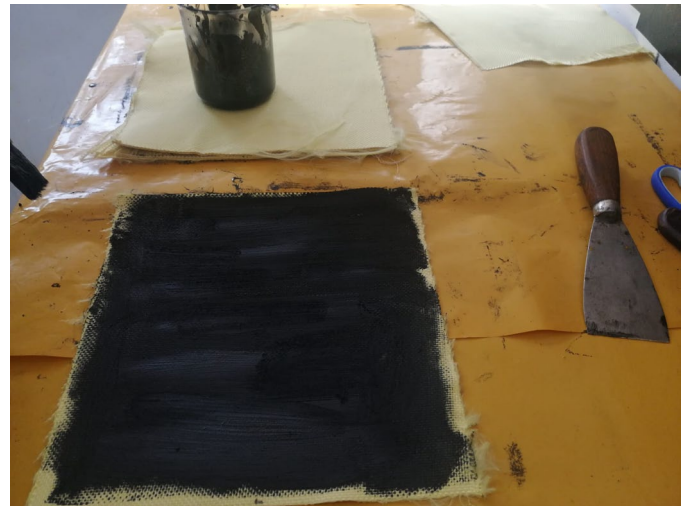
Fig. 4. Application of graphene nanopowder and epoxy resin
