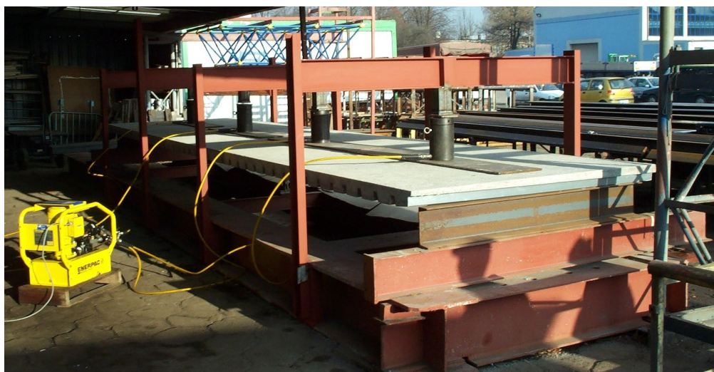
Fig. 3. Girder model on the test bench
