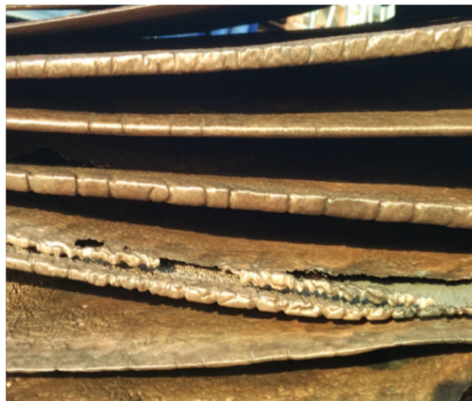
Fig. 1. Anode copper with anodic passivation
