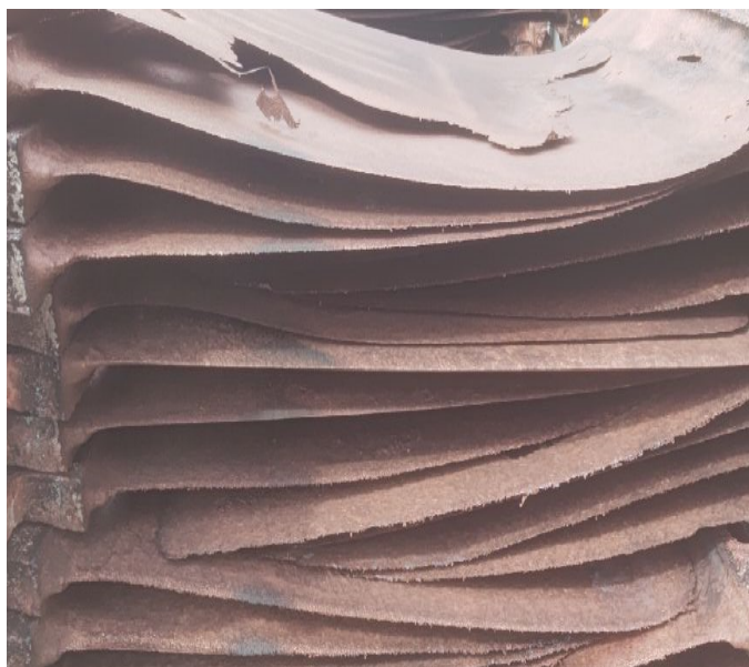
Fig. 2. Anode copper without anodic passivation
