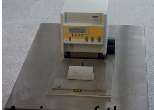
A view of the sample cooler
