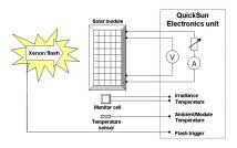
Fig. 1. The scheme of the measurement system - simulator for
