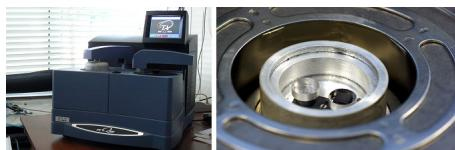
**DSC Q1000 TA Instruments:** a flux type calorimeter, temp. range **-170 - +400 °C**, heating rates 0.5 - 50K/min, liquid nitrogen (LNCS)/compressed air cooling systems, temperature modulation technique (MDSC).
