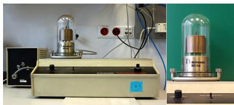
**DSC DuPont 910:** a flux type calorimeter of simple construction, temp. range **+25 - +700 °C**, heating rates 0.1 - 50K/min, gas nitrogen/ballistic cooling systems, controlled path for the inert gas.
